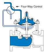
**Tight Closing Operation** When pressure below the diaphragm is relieved and operating pressure is applied to the cover chamber, the valve closes drip-tight.
