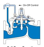
**Full Open Operation** When pressure in the cover chamber is relieved to a zone of lower pressure, the line pressure at the valve inlet opens the valve, allowing full flow.
