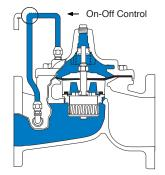
**Tight Closing Operation** When pressure from the valve inlet is applied to the cover chamber, the valve closes drip-tight.
