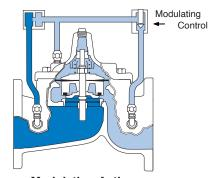
**Modulating Action** The valve holds any intermediate position when operating pressure is equal above and below the diaphragm. Using a Cla-Val "Modulating" Control will allow the valve to automatically compensate for line pressure changes.
